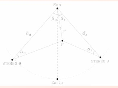
$$\tan \beta = \frac{P \sin(\alpha_A + \gamma_A) - \sin(\alpha_B + \gamma_B)}{P \cos(\alpha_A + \gamma_A) + \cos(\alpha_B + \beta_B)}$$
