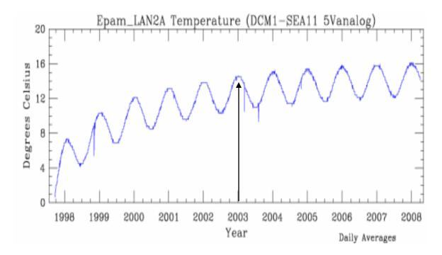
Increase in temperature is due to the degradation of the thermal blanket and not the solar cycle
