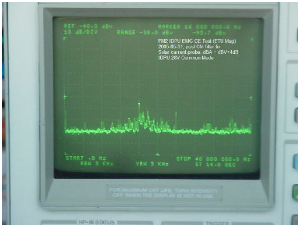
FM2 IDPU Common Mode Conducted Emissions after fix
