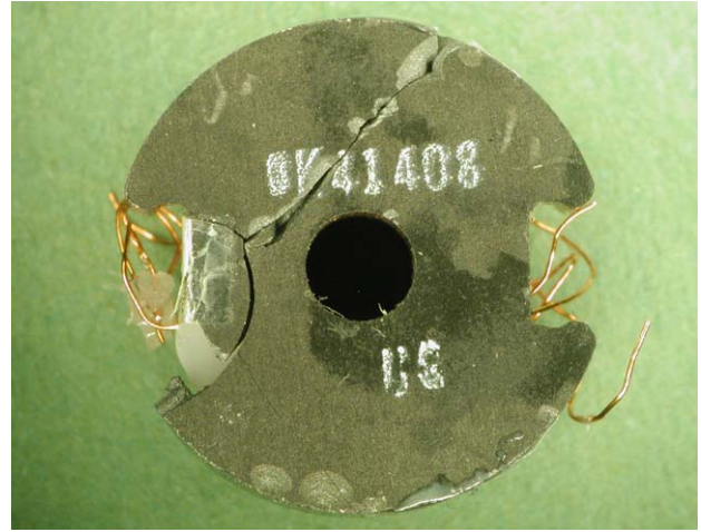
Figure 6. External photo of damaged transformer. Note cracks.
