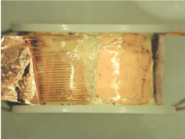
Figure 9. The copper tape is peeled back in this image, exposing a section of the outer winding.
