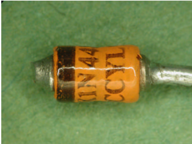
Figure 5. A side view of the 1N4480 diode. One lead was clipped close to the body during removal from the board. Curve tracer testing found the device was shorted.
