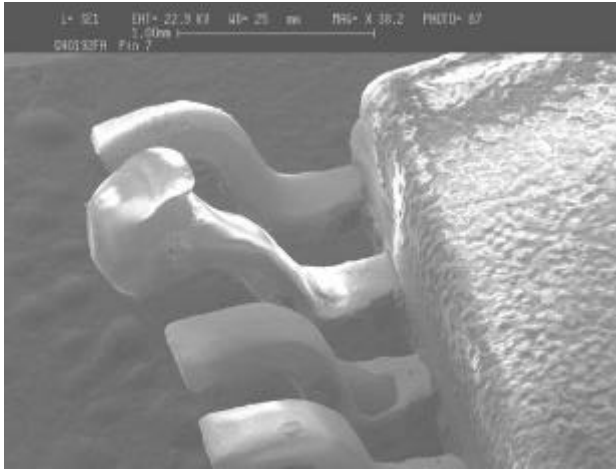
Figure 9. A tilt SEM view of Pin 7 reveals a large glop of solder on the end of Pin 7, the bottom of which appears to have two surfaces as seen in the image at right.
