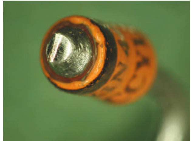
Figure 6. This end of the diode view shows a glass body under the paint.
